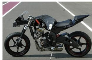
The days when we dreamt that a stock, super sport 600 might break 100 wheel horsepower are not so far behind us, but the R6 takes us into a new era. With a fully believable 133 horsepower delivered at 14,500 rpm (including RAM air effect -- at the crank), this new R6 should deliver rear wheel horsepower equivalent to the healthiest stock 750cc machine available just a few years ago.
