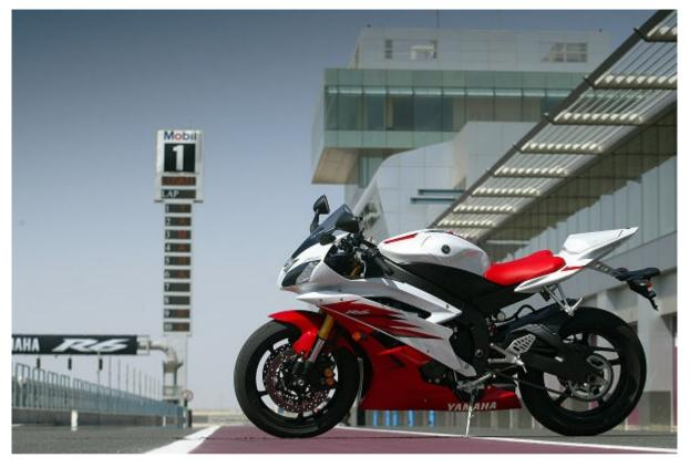
Frame geometry is aggressive with a wheel base of 54.3 inches, a rake of 24 degrees and trail of 3.8 inches.
