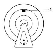
b. Turn the front wheel 90° so that the heavy spot is positioned as shown.
