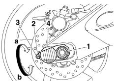
d. Tighten the wheel axle nut to specification.
