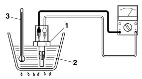
b. Immerse the air temperature sensor "1" in a container filled with water "2".
