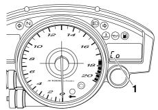
4. After selecting "Co", simultaneously press the "SELECT" and "RESET" buttons for 2 seconds or more to active the CO adjustment mode.
