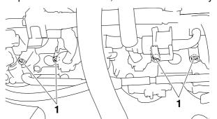
c. Using the throttle body that has the bypass air screw with a white paint mark as the standard, turn the bypass air screws without white paint marks in or out to the adjust the other throttle bodies.
