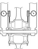
e. Measure the deflection 1.5 mm (0.06 in) below the edge of the brake disc.
