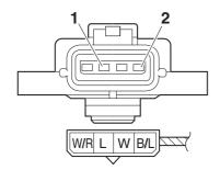
b. Measure the throttle position sensor (for throttle cable pulley) maximum resistance.
