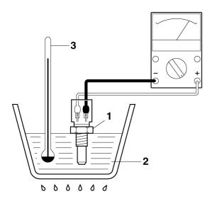
b. Immerse the coolant temperature sensor "1" in a container filled with coolant "2".
