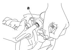
b. Remove the brake caliper piston seals.
