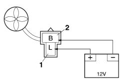
c. Measure the radiator fan motor movement.
