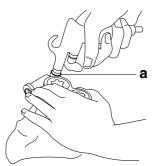
b. Remove the brake caliper piston seals.
