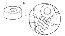
d. Calculate the sum of the values obtained in steps (b) and (c) to determine the required valve pad thickness and the valve pad number.
