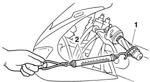
d. Hold the spring gauge at a 90° angle from the handlebar, pull the spring gauge, and then record the measurement when the handlebar starts to run.
