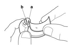
c. Put a piece of Plastigauge<sup>®</sup> "1" on the crankshaft pin.
