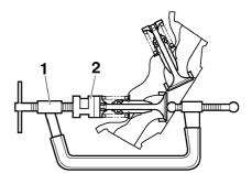
To secure the valve cotters onto the valve stem, lightly tap the valve tip with a soft-face hammer.
