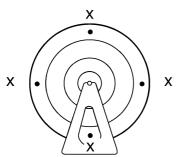
b. If the front wheel does not remain stationary at all of the positions, rebalance it.
