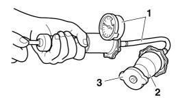
b. Apply the specified pressure for ten seconds and make sure there is no drop in pressure.
