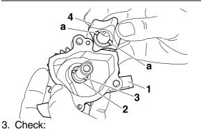
Oil pump operation Refer to "CHECKING THE OIL PUMP" on page 5-53.
