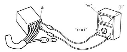
The switches and their terminal connections are illustrated as in the following example of the main switch.
