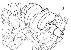
e. Install the crankshaft journal lower bearings "1" into the lower crankcase and assemble the crankcase halves.
