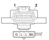
b. Measure the throttle position sensor (for throttle valves) maximum resistance.
