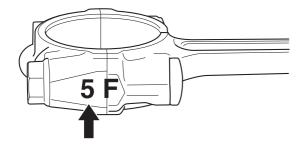
For example, if the connecting rod  $P_1$  and the crankshaft web  $P_1$  numbers are 5 and 1 respectively, then the bearing size for  $P_1$  is:
