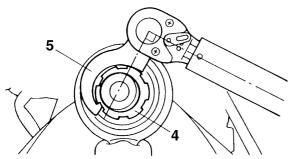
c. Loosen the lower ring nut completely, then tighten it to specification.
