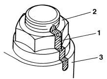
c. Tighten the connecting rod nuts further to reach the specified angle 175°–185°.
