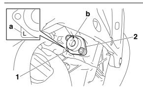
6. Rotate the crankshaft a few times to release the timing chain tensioner rod.
