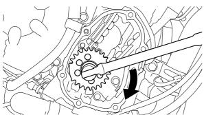
b. When piston #1 is at TDC on the compression stroke, align the TDC mark "a" on the pickup rotor with the crankcase mating surface "b".
