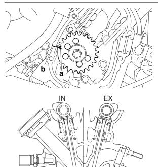
c. Measure the valve clearance with a thickness gauge "1".
