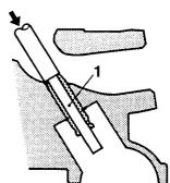
b. Install the new valve guide with the valve guide installer "2" and valve guide remover "1".
