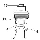
n. Remove the rod holder and fork spring compressor.
