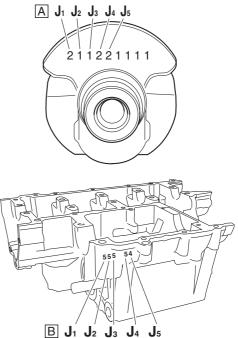
For example, if the crankcase  $J_1$  and crankshaft web  $J_1$  numbers are 6 and 2 respectively, then the bearing size for  $J_1$  is:
