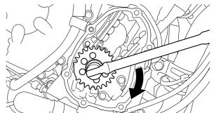
b. When piston #1 is at TDC on the compression stroke, align the TDC mark "a" on the pickup rotor with the crankcase mating surface "b".
