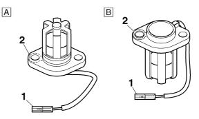
b. Measure the oil level switch resistance.
