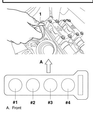
d. To measure the valve clearances of the other cylinders, starting with cylinder #1 at TDC, turn the crankshaft clockwise as specified in the following table.
