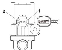
c. Measure the air induction system solenoid resistance.
