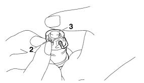
c. Hook the clip "4" to the timing chain tensioner rod "3".
