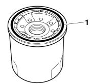
e. Tighten the new oil filter cartridge to specification with an oil filter wrench.
