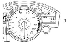
1. Odometer/tripmeters/fuel reserve tripmeter/stopwatch
