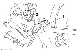
4. Install:Swingarm pivot shaft ring nut "1"
